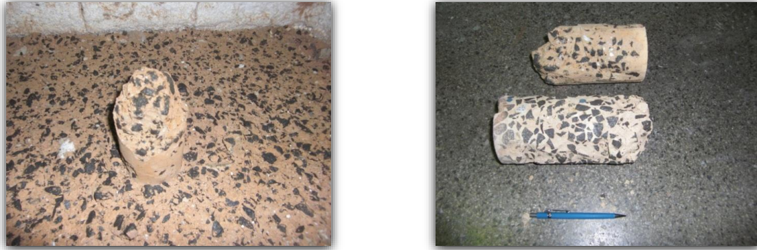
Figure 15. Small cylindrical unreinforced HSCC specimens partially disintegrated after fire testing; they had been placed together with the large prototype column.
