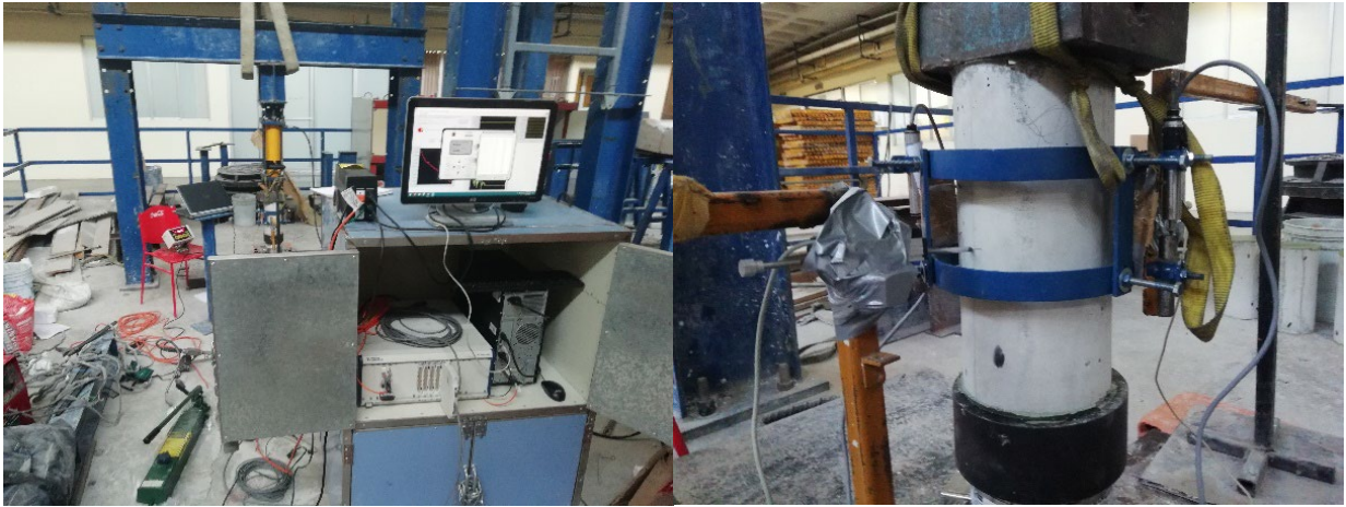
Figure 2. Instrumentation setup for short-term creep tests by sustained compression.
