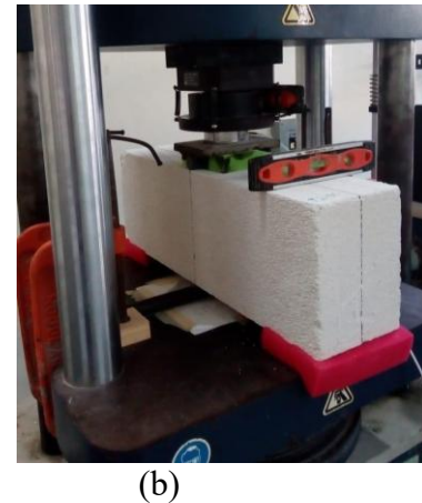
Figure 1. Test to determine the splitting tensile strength of AAC. (a) Test setup. (b) Test view
