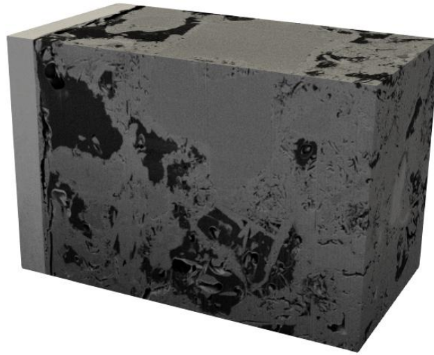
Figure 4. FIB-SEM nanotomography of the SCI pore structure (Ruffray et al. , 2023).
