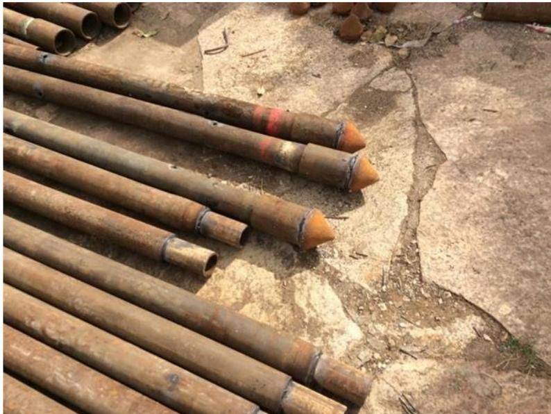
Figure 10. Focus on the Manessmann tubes with a diameter of 73 mm. Injection drilling and driving azuches are observed without vibration transmission to the surrounding soil.
