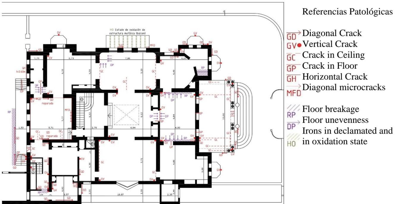
Figure 3. Pathology survey at ground floor level.
