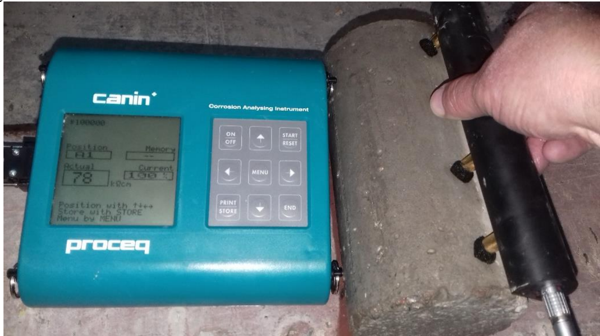
Figure 3: Resistivity measurement procedure. CANIN device. Wenner probe.
