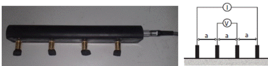
Figure 2: Wenner probe used. Measurement scheme.
