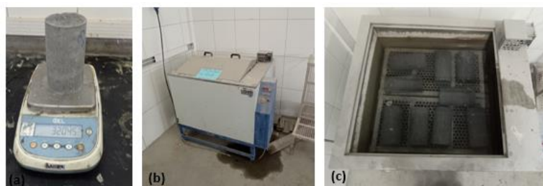
Figure 3. Steps for carrying out the absorption test and void ratio
