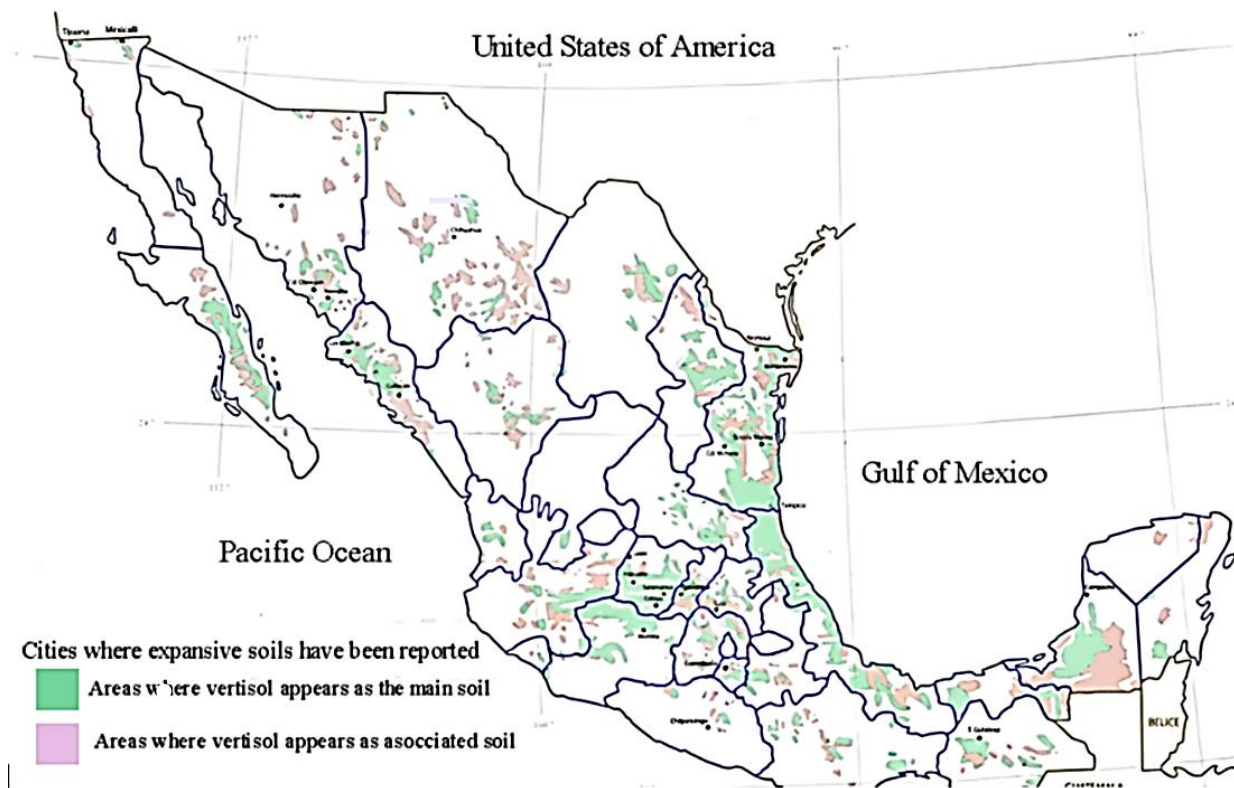
Figure 2. Potential areas of expansive soils in the Mexican Republic (Zepeda and Castañeda, 1989).
