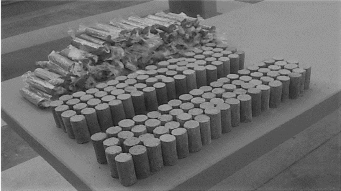
Figure 10. 144 specimens of clay mixtures with different stabilizers ready for the triaxial test UU (Miranda, 2017).
