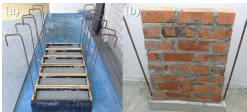
Figura 2. (a) Base de pared (b) Pared terminada
