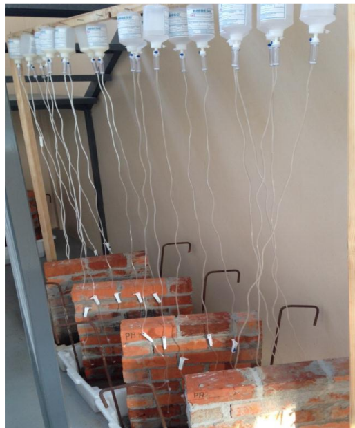
Figure 4. Application of waterproofing products.
