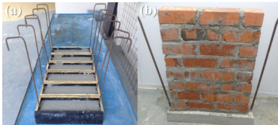
Figure 2. (a) Base of the wall and (b) Finished wall.
