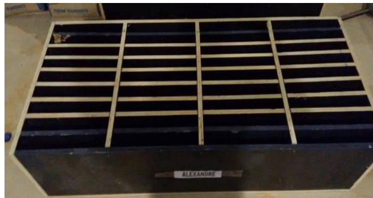
Figure 4. Rectangular mold capable of producing 36 specimens.
