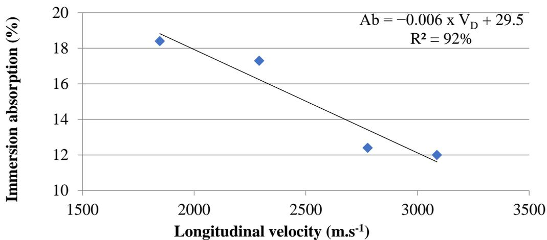
Figure 3. Regression model between immersion absorption and longitudinal velocity.
