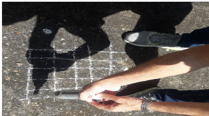
Figure 7. Carrying out the sclerometer test
