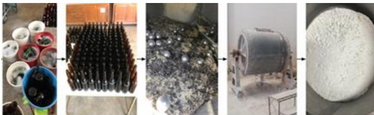
Figure 1. Recycled glass powder processing.
