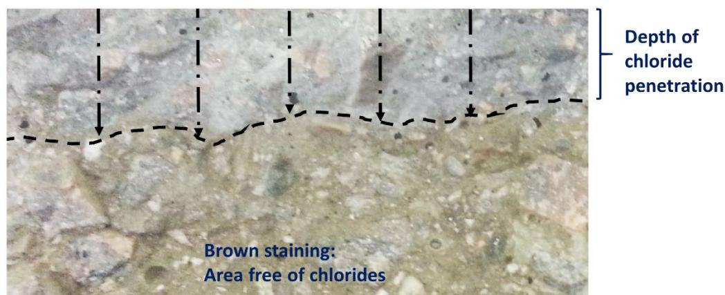
Figure 7. Illustration of the contrast obtained with the application of the colorimetric method to determine the depth of penetration of chlorides, using a spray of a solution of NaOH and one of AgNO<sub>3</sub>.
