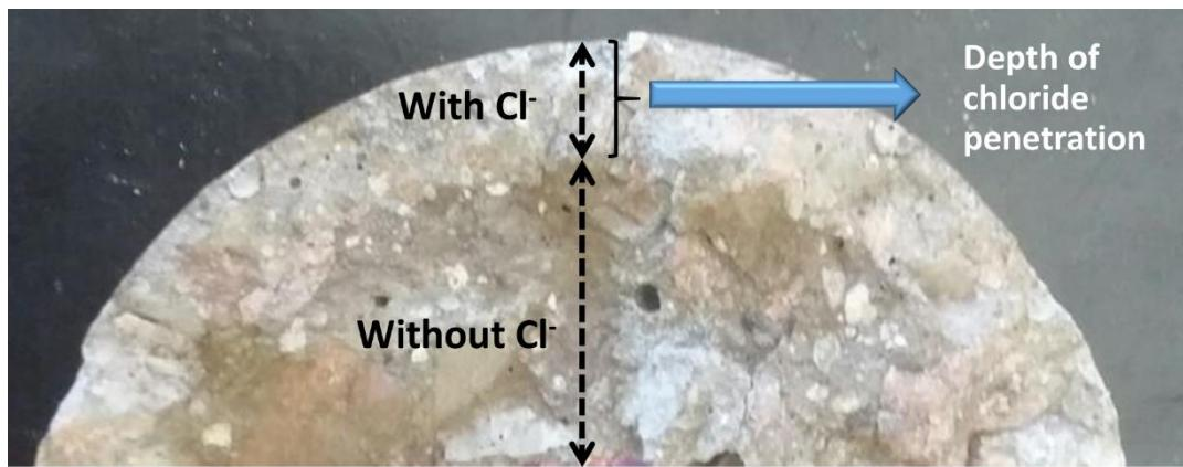
Figure 1. Chloride penetration depth measurement by visual colorimetric method by spraying an aqueous solution of 0.1 M AgNO<sub>3</sub>.
