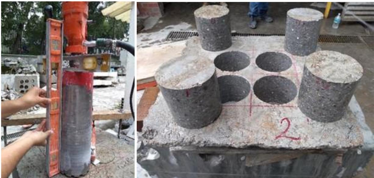
Figure 10. Specimens removal for the Barcelona Test.
