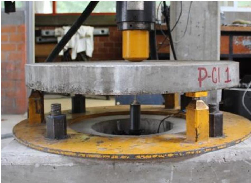
Figure 7. Round panel test setup, ASTM C1550
