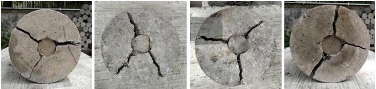
Figure 12. Cylinders typical failure mode, Barcelona Test.
