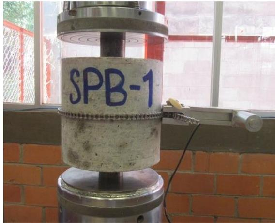
Figure 11. Double punching test, configuration, UNE 83515
