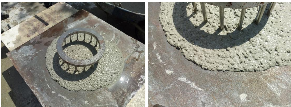
Figure 5. Detail of passing skill test through the J ring, performed in the laboratory during the dosage study.
