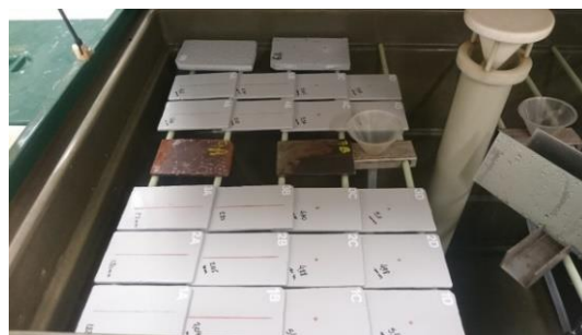
Figure 6. Specimens in the salt chamber before exposure to the mist (Ribeiro Filho, 2018).
