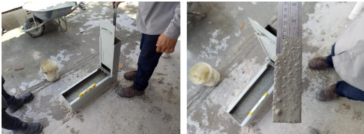
Figure 4. Detail of passing skill test through box L, performed in the laboratory during the dosage study.
