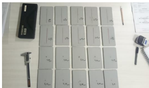
Figure 5. Specimens with experimentally damaged paint (Ribeiro Filho, 2018).
