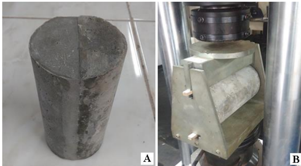
Figure 3. (A) Test body used to determine the adhesion between the repair and the concrete; (B) Test to determine the adhesion between the repair and concrete by diametral compression.
