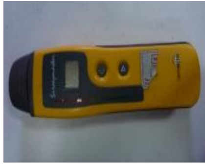
Figura 6. Higrômetro Protimeter Surveymaster SM.
