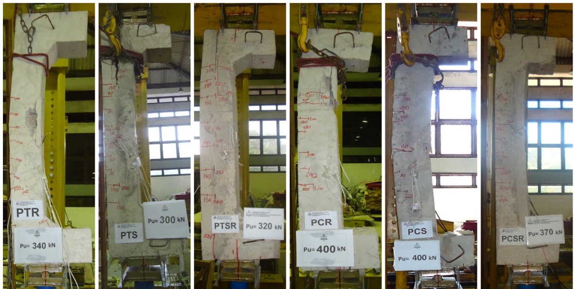
Figure 10. Columns after failure.
