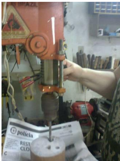
Figure 4. Drilling tests with fixed drill.
