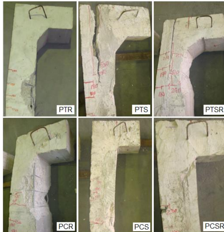
Figure 11. Details of columns after failure.
