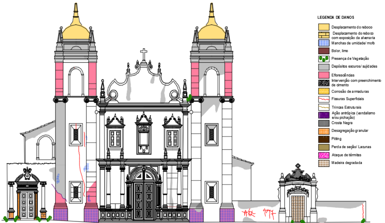
Figure 10. Damage Map of the North Façade of the Carmo Church. Source: Authors.
