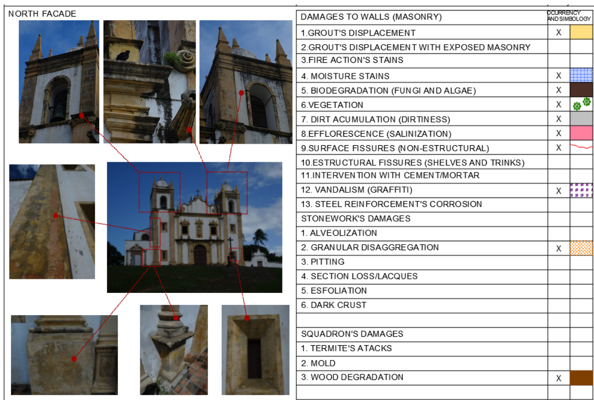
Figure 6. Damage identification form for the north façade of the Carmo Church. Source: Authors.
