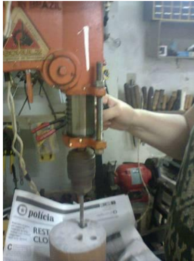
Figure 4. Drilling tests with fixed drill.
