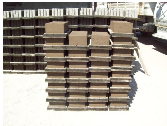
b) stowage and curing of units
