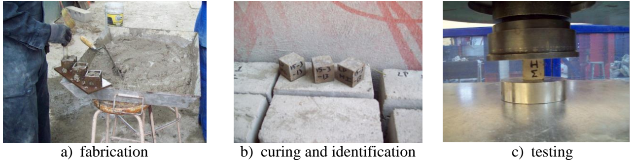
Figure 10. Building, curing and testing of mortar cubes
