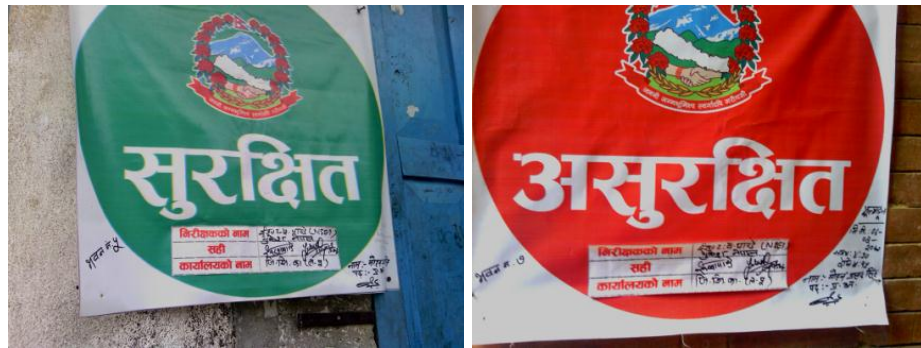
Strikers: Safe and Unsafe Category of Buildings Figure 2. Rapid Vulnerability Assessment
