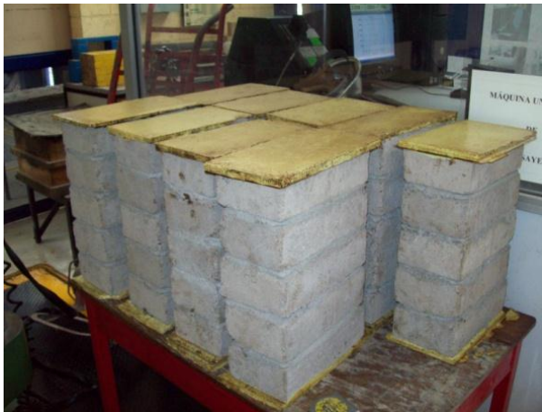
a) Preparation of prisms for testing
