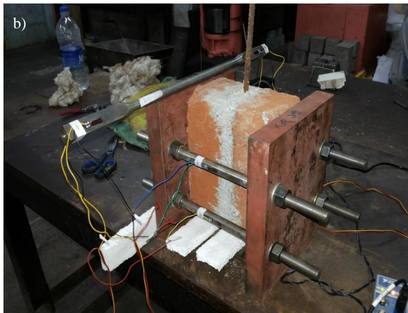
Figure 2. (a) Sample held in position (b) Pull-out Test set-up
