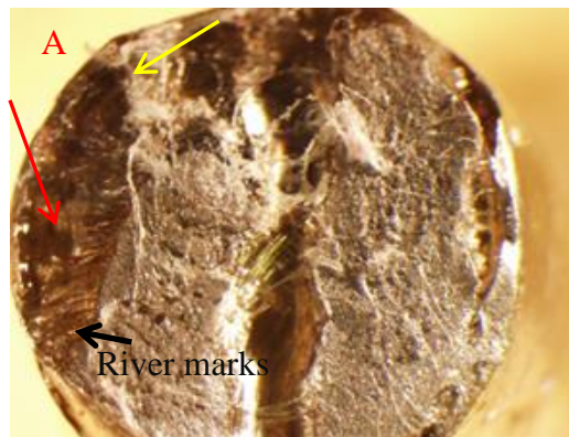
Figure 11A. Fracture of the specimen with single bevel specimen with buttering. Lack of fusion (red arrow) and blowholes (yellow arrow) are observed on the fracture.
