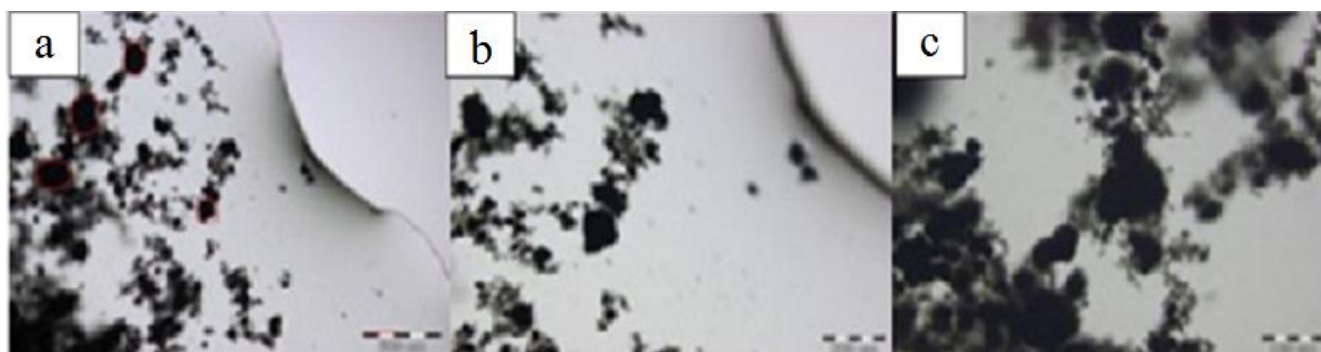
Figure 6. Sample SM 2 - powder CNT dispersed in water and a polycarboxylate admixture (Tec Flow 8000 - at 2%).
