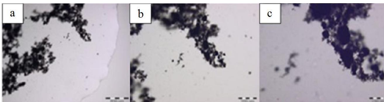
Figure 15. Sample SM 11 - powder CNT dispersed with Arabic gum and water.
