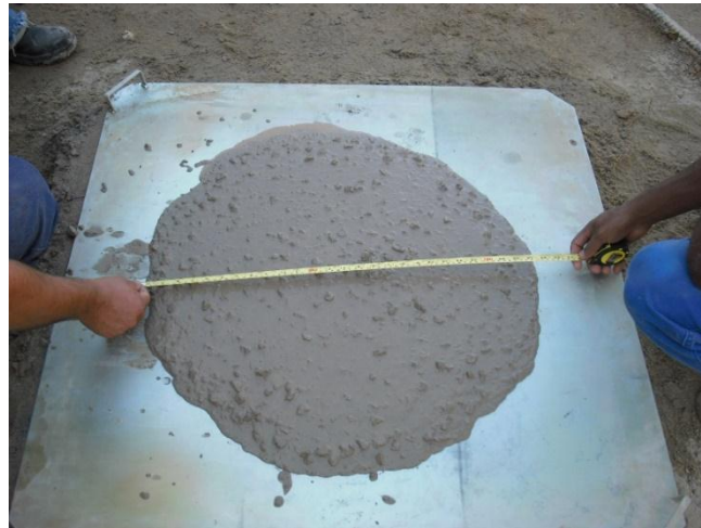
Figure 9. Measurement of concrete flow.
