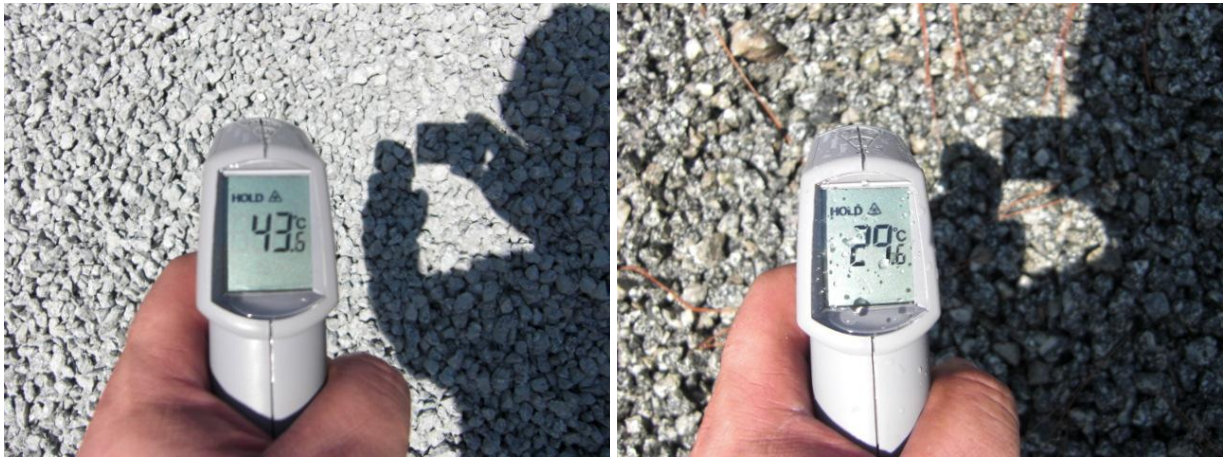
Figure 7. Register of coarse aggregate's temperature before and after the being water-sprayed at Ready-mix Company batching plant.
