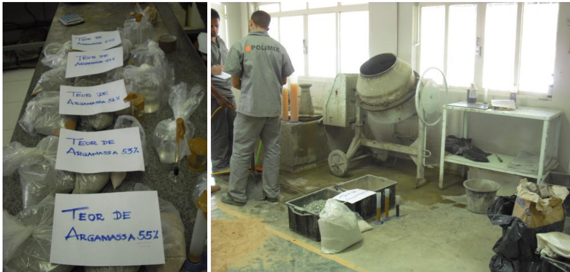
Figure 2. Mixes with different mortar content.
