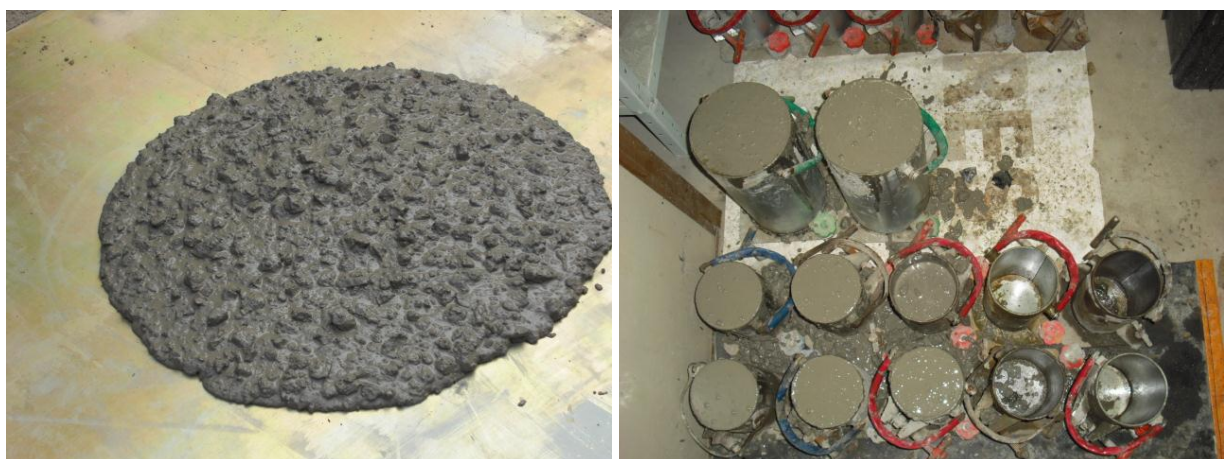
Figure 4. Flow test and specimens being cast for compressive strength tests.
