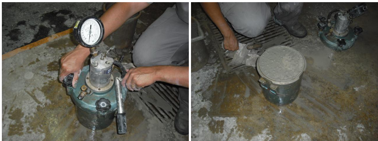
Figure 3. Trapped air contents and specific apparent gravity measurement.
