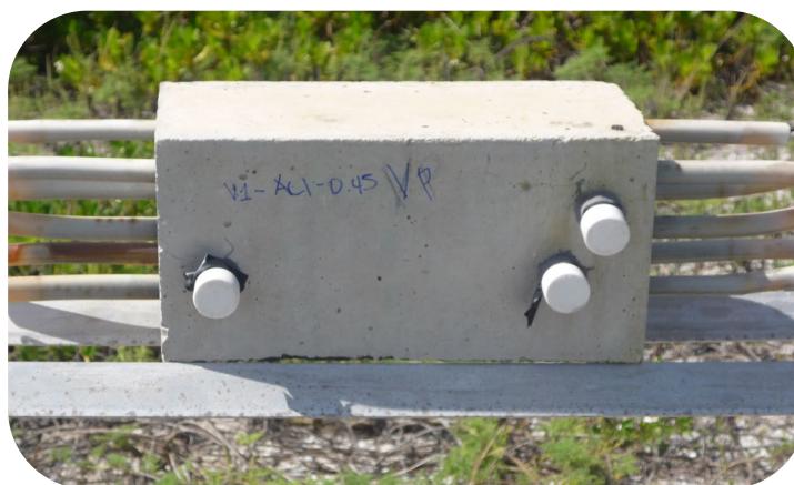
Figure 1. Specimen and its exposure scheme; the major coating is in the lower bed.
