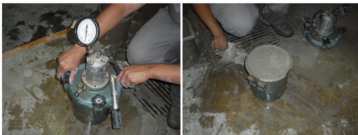
Figure 3. Trapped air contents and specific apparent gravity measurement.
