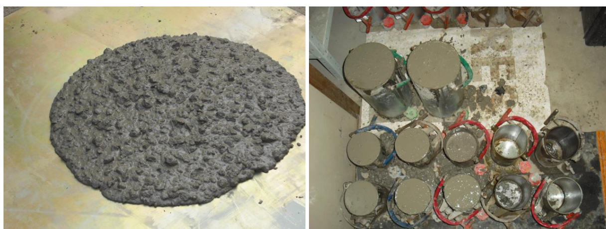
Figure 4. Flow test and specimens being cast for compressive strength tests.
