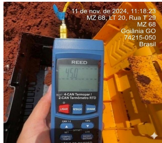
Figure 9. Temperature record of T = 45,0\text{ }^{\circ}\text{C} after 72 hours in the test block.
