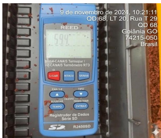
Figure 7. Temperature record of T = 59,4\text{ °C} after 24 hours in the test block.
