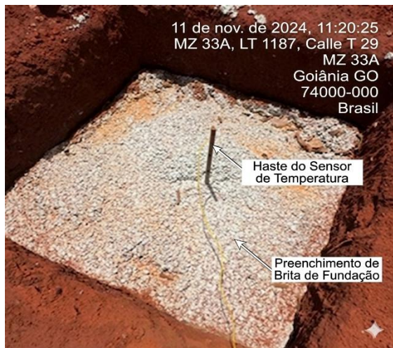
Figure 8. Record of the test block after 72 hours.
