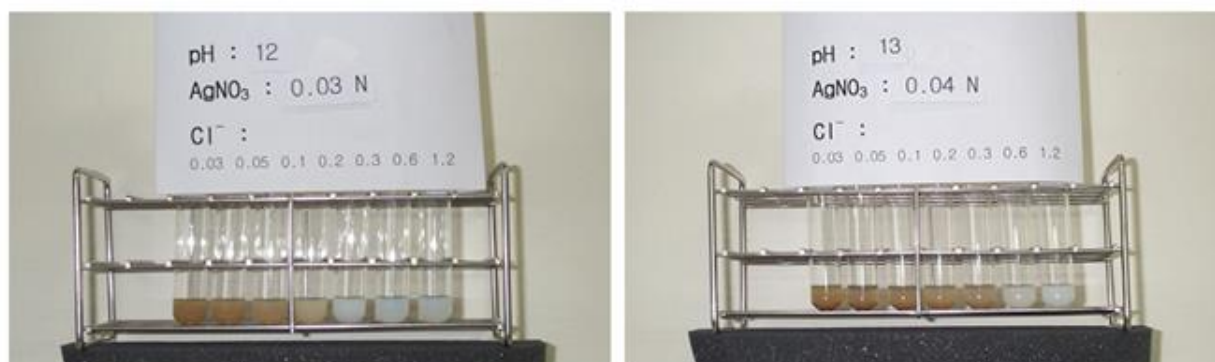
Figure 7. Analysis of the influence of pH on the color change (KIM et al. , 2013).
