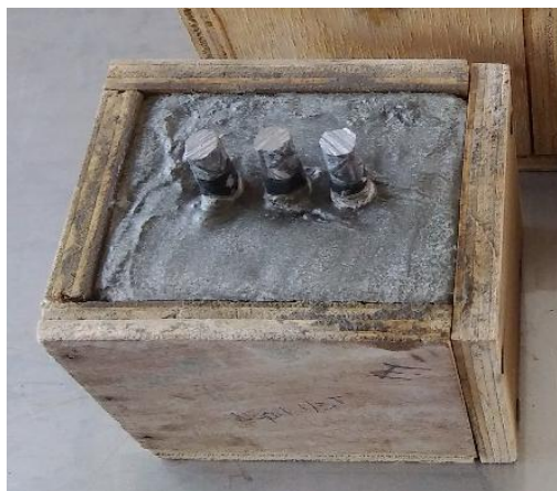
Figure 2. Concrete block with three reinforcing steel bars.
